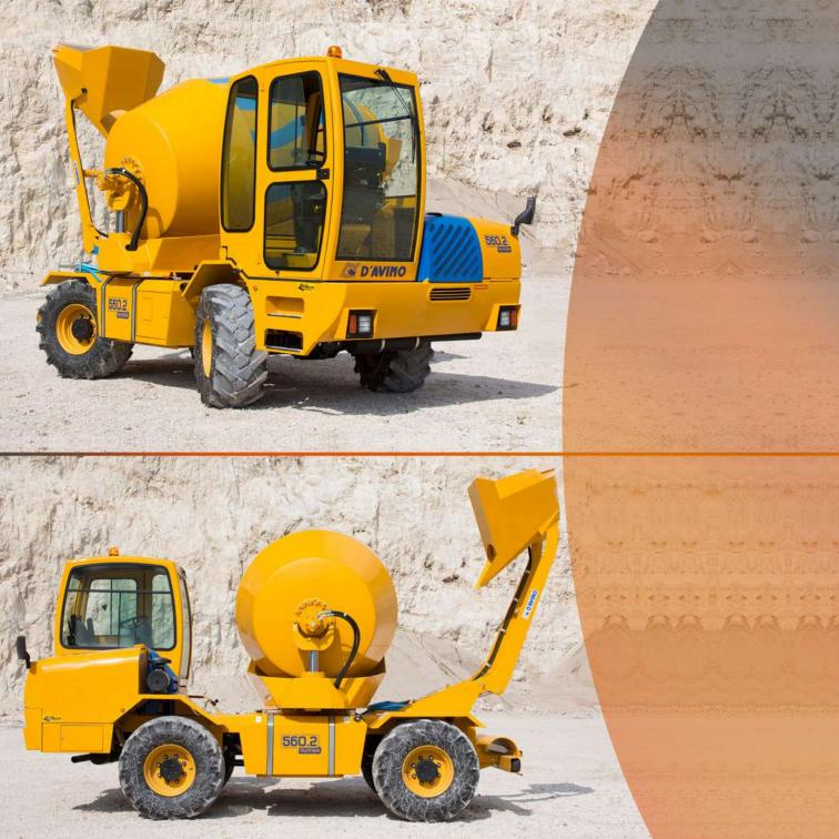
**DESCRIPTION** (UNI 10929:2011) Self-Loading Concrete Mixer – Concrete net output: 4,5 m3 (5.25 cubic yards) class S1 - Rear loading – Trilateral unloading (slewing 180°) - N.4 wheel steering/drive – Loading by rigid bucket
