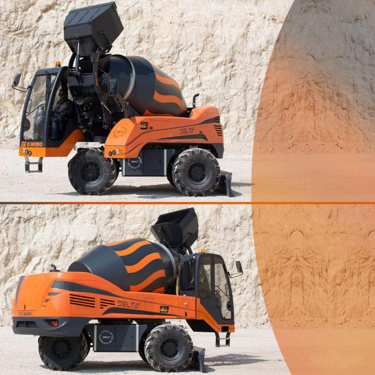
**DESCRIPTION** (UNI 10929:2011) Self-Loading Concrete Mixer – Net output 4,5 m3 (5.90 cubic yards) (\$1 class) – Load and cast through the full 360° (continuous rotation) – 4 wheel driving and steering – Articulated bucket integral with rotating frame – Cab integral with 360° rotating frame (continuous rotation)
