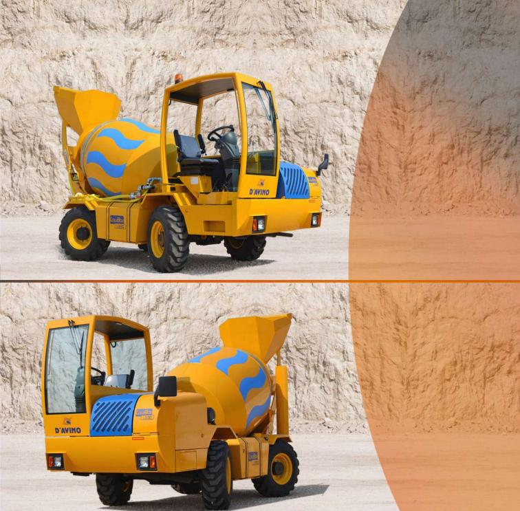
DESCRITPION (UNI 10929:2011) Self-Loading Concrete Mixer – Concrete net output 2,8 m3 (3,7 cubic yards) class S1 – Rear loading / unloading - N.4 wheel steering/drive ← Loading by rigid bucket
