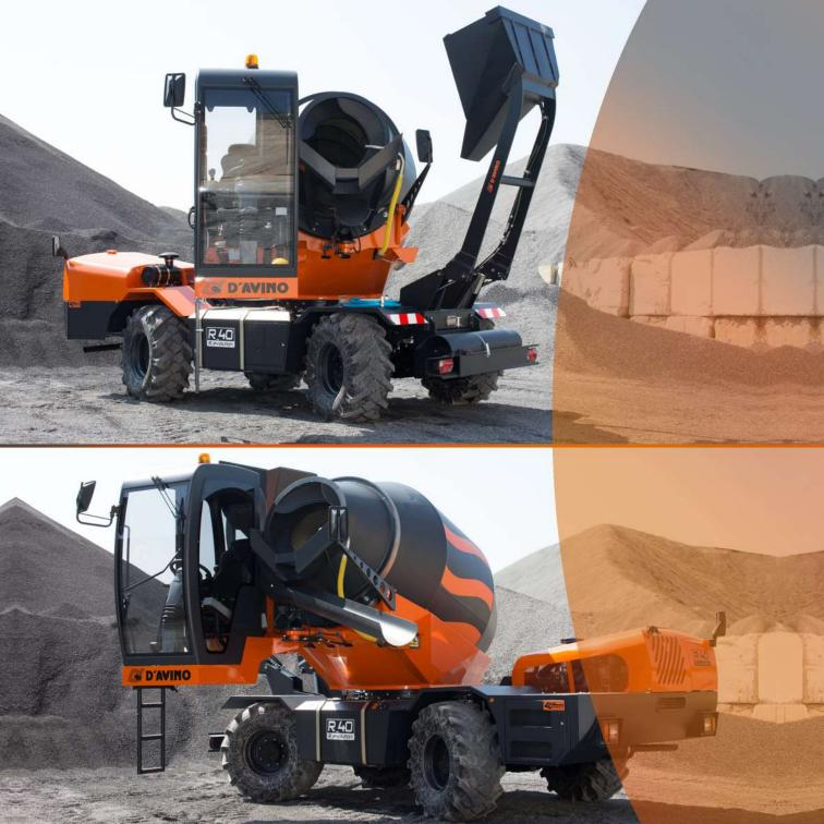
**DESCRIPTION** (UNI 10929:2011) Self-loading concrete mixer - Concrete net output: 4,5 m3 (class S1) - Front loading - Trilateral unloading (slewing 315°) - N.4 wheel steering/drive – Loading by rigid bucket - Cab welded to the rotating drum and slewing at 315°
