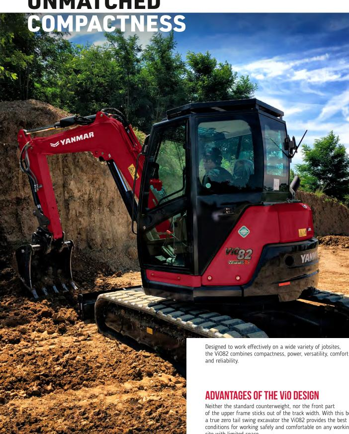
Neither the standard counterweight, nor the front part of the upper frame sticks out of the track width. With this being a true zero tail swing excavator the ViO82 provides the best conditions for working safely and comfortable on any working site with limited space.
